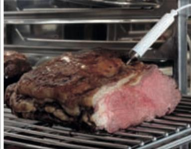
Multipoint cooking probe (Lev. 3), singlepoint (supplied as standard in Lev. 2, optional in Lev. 1) and vacuum (optional) = controlling product core temperature in all conditions.
